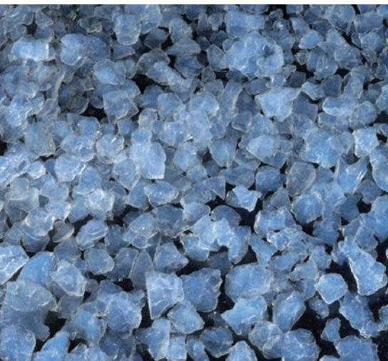
Nanogel pellets transmit light and act as insulators.
